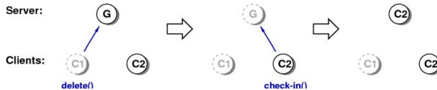
Figure 4: One client deletes his local copy (C1) and the global version (G) of a specific part while a second client still holds another (writeable) copy (C2). Afterwards, the second client writes back his copy (C2) and “undos” the previous operation—an inconsistency occurred.
