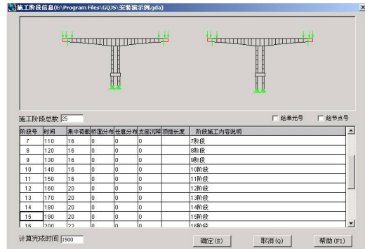
Fig.6 Construction Stage Information
