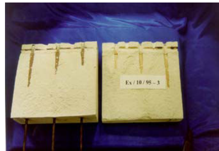
Abb. 4.2.4.10 d_{sA} 10mm; e=95 mm
