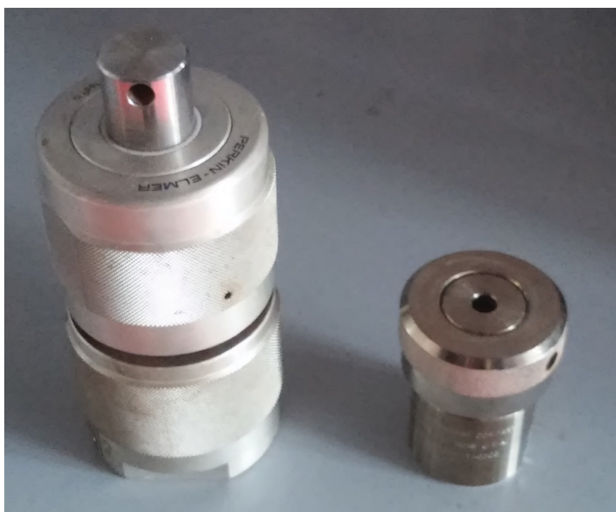
Fig. S1: Reactor vessels utilized in MOF syntheses: (Left) 110 mL Perkin Elmer acid digestion bomb for MIL-144. (Right) 23 mL Parr acid digestion bomb for JUMP-2.
