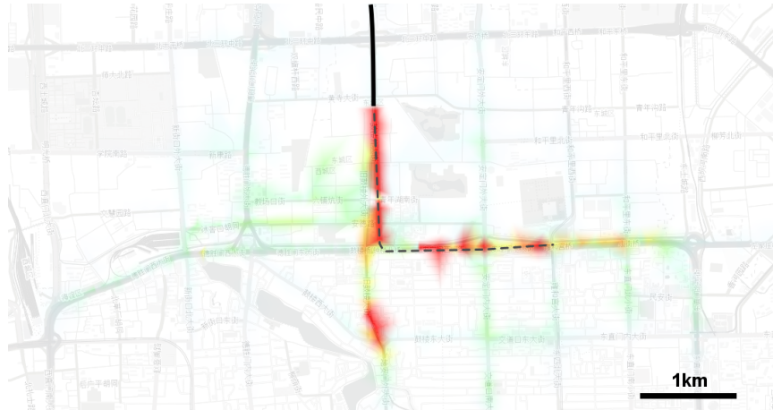
Figure 6.19: Exemplary prediction of a single taxi drive. The observation is shown as a solid black line and the path for the next ten minutes is plotted as a dashed line. The probability distribution is shown in colors ranging from turquoise (low probability) to red (high probability). Since it is not possible to show the distribution for every time step in a single picture, the accumulated distribution is shown from t = 0 to t = 600s to depict the most probable paths the car might take in that time period. As can be seen, the prediction correctly assumes a left turn (east) at the crossing in the middle while still maintaining a slightly lower probability for heading further south. The final position of the car at t = 600s conforms with the predicted probability distribution, too. Paths along the side roads are also considered and taken into account with a low probability. 1
