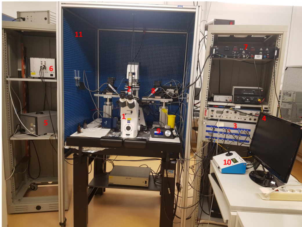
Figure 13: Setup for patch-clamp electrophysiology and photometry: 1-inverted microscope, 2-viewfinder, photo-diode, and camera, 3-patch-clamp amplifier, 4-computer monitor, 5-polychrome-V monochromator, 6-Fluorescence detection unit for single emission (FDU-SE), 7-temperature control device, 8-patch pipette holder, 9-micromanipulator, 10-microscope stage controller, and 11-Faraday cage.
