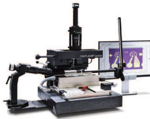
Fig. 2.6. Fineplacer lambda from Finetech GmbH & Co. It contains two cameras (left and over the device) to allow fine adjustments, an operating plate with the pick-up tool and a hot plate; and a computer to program temperature profiles [18].
