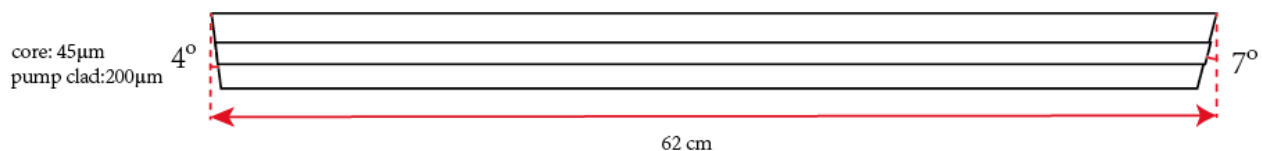
Figure 7.27 Schematic of rod fiber 854b
