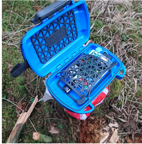
Figure 4.12: Fully assembled Raspberry Pi node with casing
