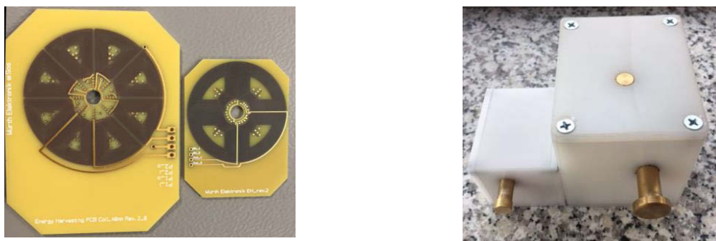
Figure 3: Comparison of miniaturized and previous harvester : (a) coil systems and (b) completed harvesters
