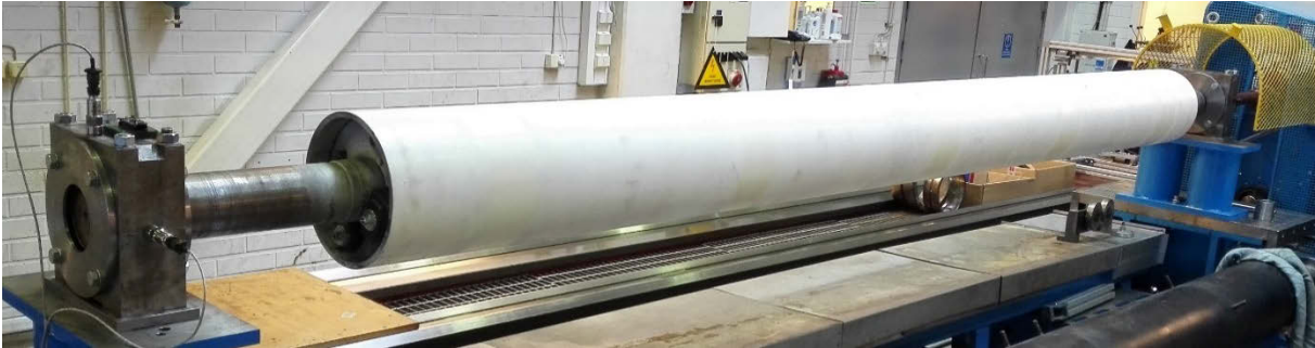
Figure 2 Test rotor and the measurement setup in the tending side bearing housing.
