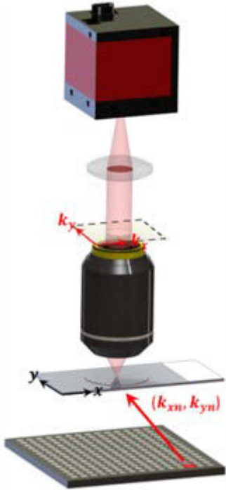
Figure 2: Classical transmission mode setup for microscopes. FPI is based on LED matrix illumination.
