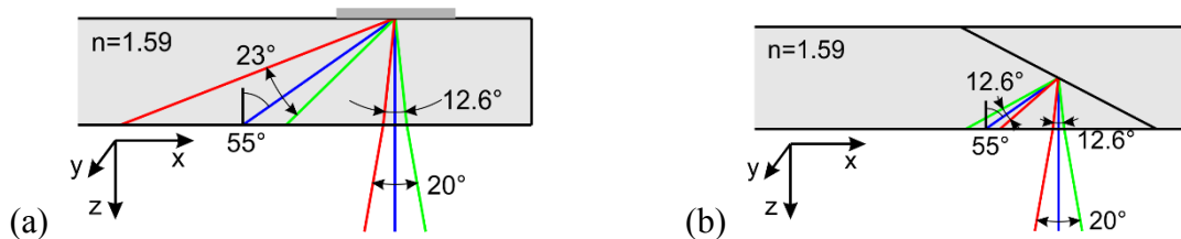
Figure 4. Comparison between the deflection at (a) a surface relief grating and (b) a slanted mirror or beam splitter. The different colors represent the chief rays for different field angles and are not related to the wavelength.
