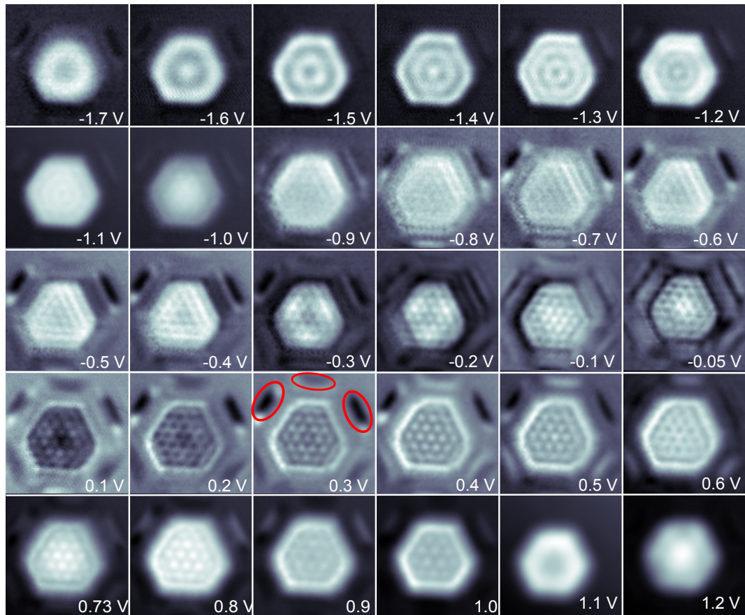
Figure A.2: Complete gallery of all dI/dV maps recorded atop an exemplary cavity buried 4 atomic layer underneath the Pb(111) surface at the indicated voltages (1 nA, 7.8 \text{ nm} \times 7.8 \text{ nm} ). The gallery is an expansion of the dI/dV maps shown in figure 4.7(a). The majority of the dI/dV maps show additional elongated structures outside of the central hexagon (red circles at 0.3 V). These modulations of the LDOS have been reported before [128] and can be attributed to electron standing waves between the crystal surface and the edges of the downward sloping Wulff construction which determines the shape of the buried cavity.
