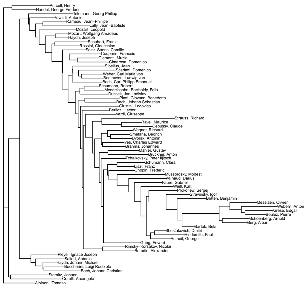
Figure 7.26. Hierarchical clustering using the minimum evolution criterion. With this method (ordinary least squares with unweighted subtrees), the branch length corresponds to the distance of nodes or items to their ancestor. The minimum evolution criterion enforces the total length of branches to be minimal.
