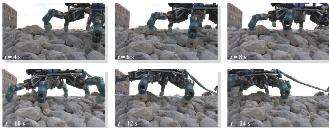
Figure 4.26: The DLR Crawler crosses a gravel field within the DLR outdoor testbed
