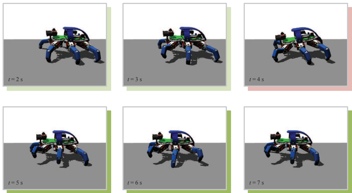
Figure 5.14: Simulation of the DLR Crawler experiencing the loss of its left front leg (L1); light green frames: the robot is fully functional, red frame: the left front leg is lost (i. e. lifted and hold in this position), green frames: the robot instantaneously adapts its gait, shifts its COG away from L1, and increases its joint stiffness settings
