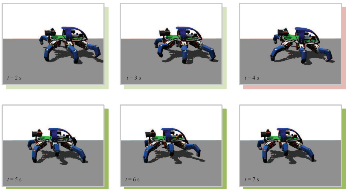
Figure C.1: Simulation of the DLR Crawler experiencing the loss of its left middle leg (L2); light green frames: the robot is fully functional, red frame: the left front leg is lost (i. e. lifted and hold in this position), green frames: the robot instantaneously adapts its gait, shifts its COG away from L1 and increases its joint stiffness settings
