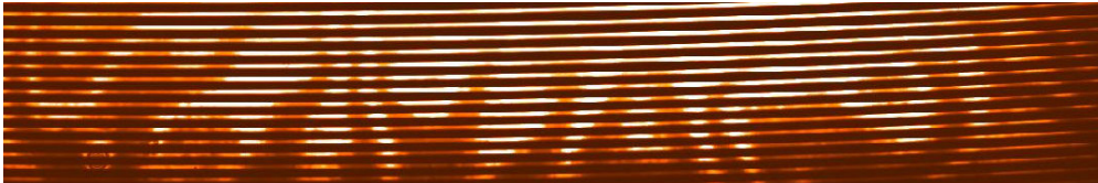
Figure 5.2: Part of a typical flat-field frame, taken with the CAFE spectrograph at the 2.2-m telescope at Calar Alto observatory.
