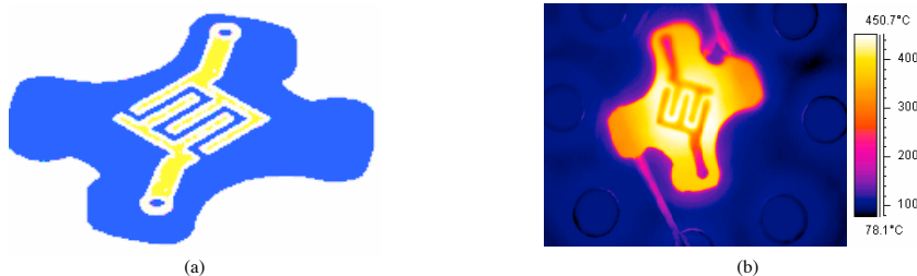
Fig. 3: The design (a) and infra-red picture of improved LTCC sensor substrate (b).
