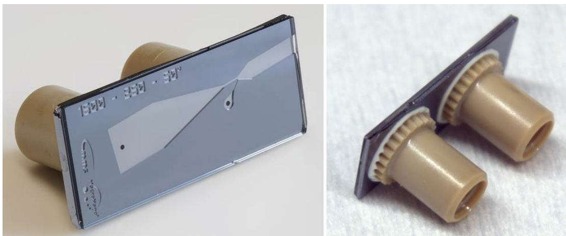
Figure 3. Photographs of the fabricated micro-Venturi injector. The microfluidic channels are etched into silicon and enclosed by a cover glass plate. The fluid connection to the chip is realized by NanoPort™ assemblies.
