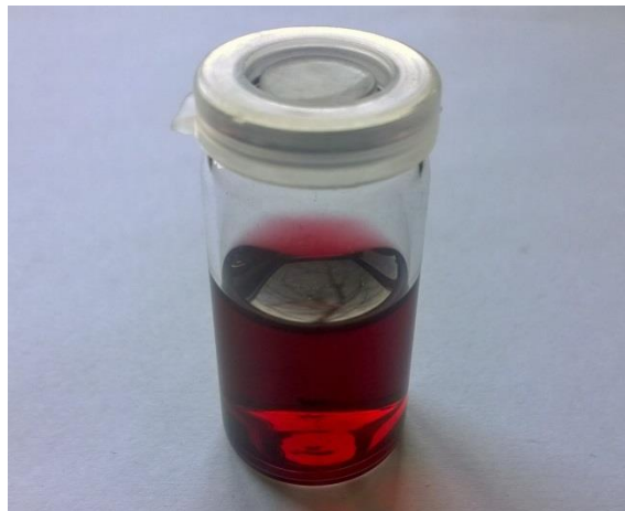
Fig. 9 The colloidal solution of gold nanoparticles prepared by means of Turkevich technique
