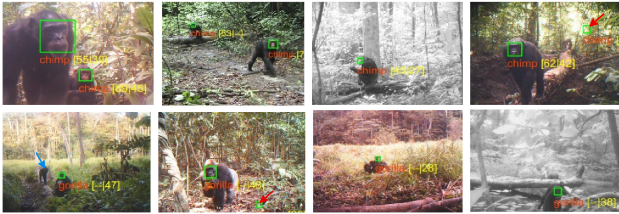
Figure 4.3.: Detection results by SHORE^{TM} of near-frontal chimpanzee and gorilla faces in their natural habitats. Detected faces are marked with green rectangles. The species is automatically assigned to every face using the detection scores of the chimpanzee and the gorilla model, respectively. Both scores are superimposed in yellow ([chimp-score|gorilla-score]). In case one detection model did not find a face, the corresponding detection score is replaced by hyphens. Although background clutter and challenging lighting conditions place high demands on SHORE^{TM} only few faces were missed (blue arrow) and few false positive detections occurred (red arrows). Image source: [113]. [I02, I03]
