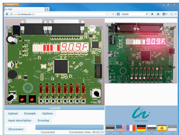
Figure 6. Web-interface of the rapid prototyping board (RIA)
