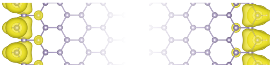
Figure 3.7: Wave-function square of the edge states with vanishing energy at X . Ge and H atoms are shown as small purple and white spheres. The center of the ribbon is omitted.
