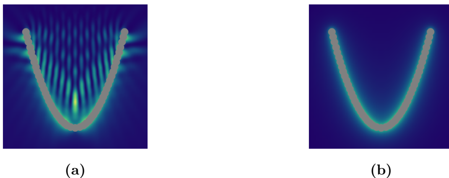
Figure 4.1: (a) Intensity of 51 spherical wave emitters (covered by gray circles) arranged on a parabola. The intensity of each emitter decays fast as 1/r^2 . The intensity in the parabola stems almost exclusively from the interference term. The frequency is chosen such that a nice interference pattern occurs. For high frequencies, the intensity concentration in the focus becomes much more pronounced such that the intensity becomes negligible everywhere except in this single spot. This can also be seen from comparison with (b) , where the same situation is shown with the interference terms left out.
