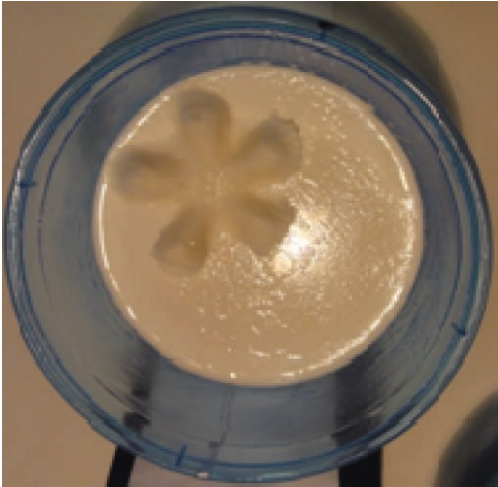
Fig. 15: Photograph of a phantom with rosette shaped tumor surrogate before casting the resist layer
