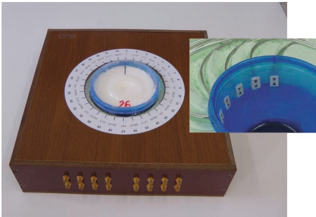
Fig. 4: Finished antenna array with inserted rotatable breast phantom and horizontal antenna arrangement before casting the contact layer
