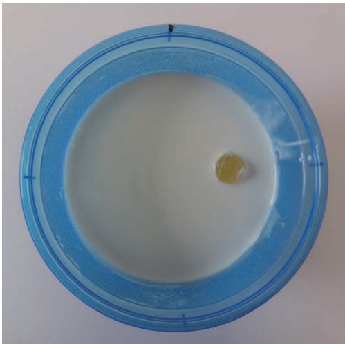
Fig. 11: Photograph of a homogeneous phantom before casting the resist layer with still visible tumor surrogate on the right side
