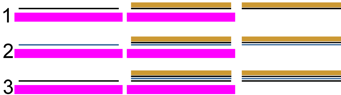
Figure 5.1.3. (1) Transfer of graphene (black line) from SiO 2 /SiO substrate (purple box) to quantifoil grid (yellow line)– graphene/grid. (2) Transfer of g-C 3 N 4 (blue line) to graphene/grid. (3) Another graphene flake is transferred to g-C 3 N 4 /graphene/grid.
