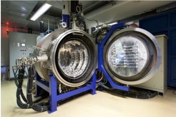
Figure 5: Diffusion bonding system
