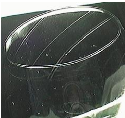
Figure 5: Photo of line corrosion
