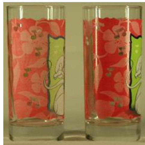
Figure 12: Glass & decor protection in consumer-test (50 x)
