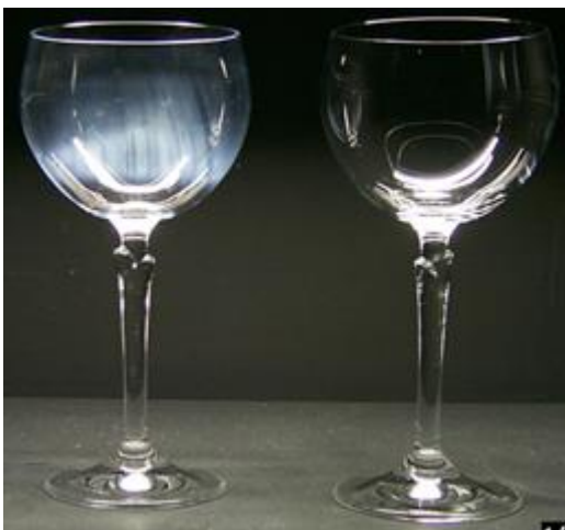
Figure 11: Glass protection in lab-test (100 x)
