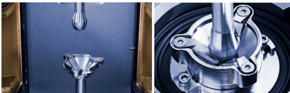
Figure 2.1: Tribological measurement for bearings, ball on three plates [1]
