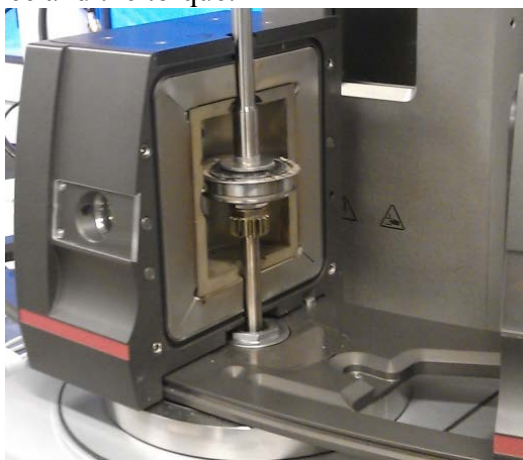
Figure 3.1: Heatable measuring system (rotatory rheometer) [2]
