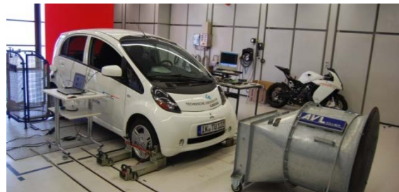
Figure 2.2: EV on a dyno test bench
