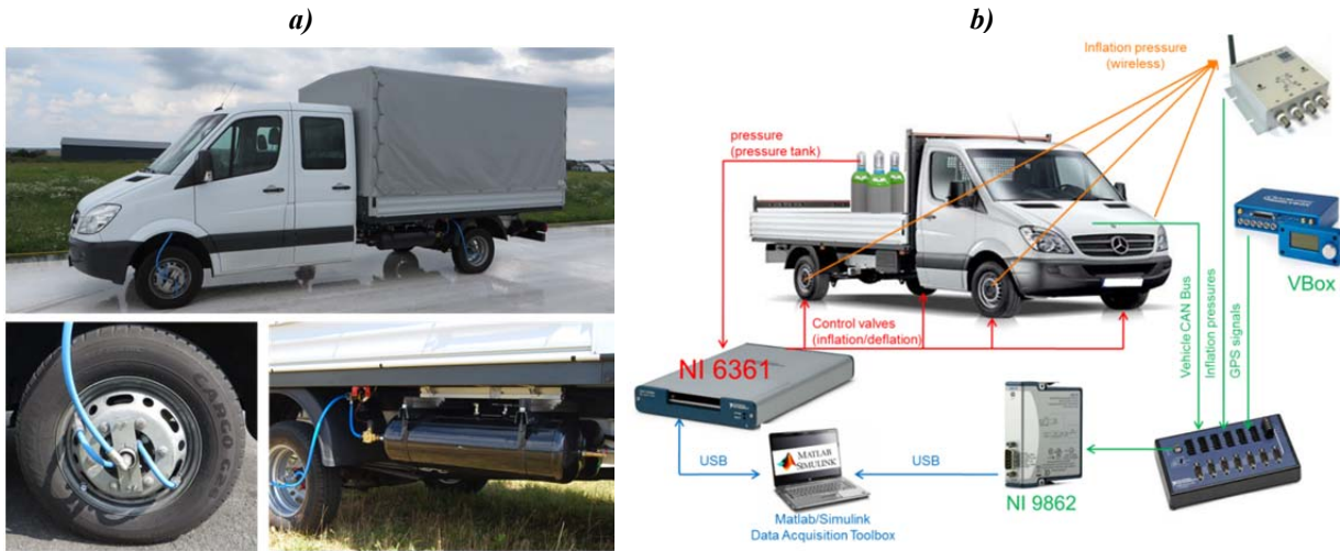
Figure 8: a) test vehicle with TPCS b) communication layout of test vehicle with TPCS
