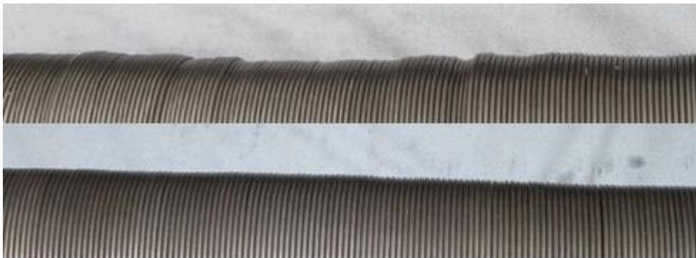
Figure 9: Comparison of two spring sections (“Wire 1” above; “Wire 2” below)
