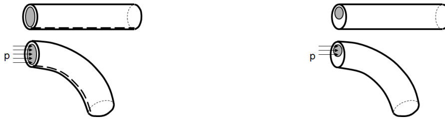
Figure 5. Schematic of bending under inner pressure. The left Image shows a silicone body embedded with a non-stretchable thin fibre in the wall and a hollow symmetrical centre core, the right Image shows an asymmetrical hollow core in the silicone carrier.
