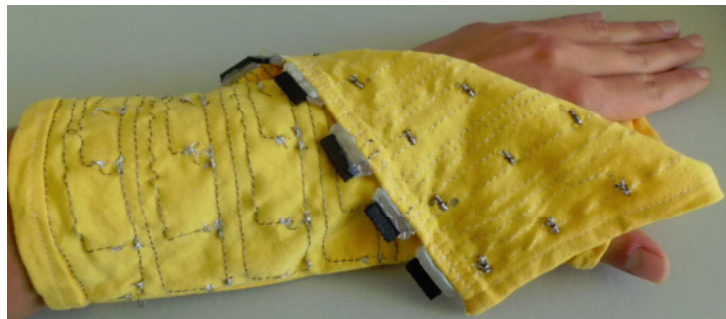
Fig. 4: Textile temperature sensor mat with 40 SMD thermistors
