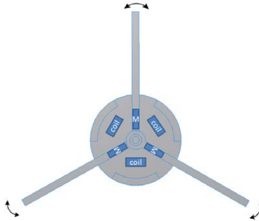
Fig. 1. A functional principle of the wheg module with electromagnetic spokes
