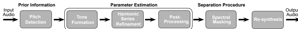
Figure 3.35.: Block diagram of the proposed tone-based solo and accompaniment separation algorithm. It has to be noted that an additional Tone Formation block has been included in the parameter estimation stage if compared to the frame-based separation method in Figure 3.1.
