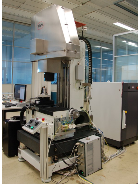
Fig. 13 Vertical setup consisting of Tilted Wave Interferometer, combined long range and X-Y-Z-positioning unit, control system and work place
