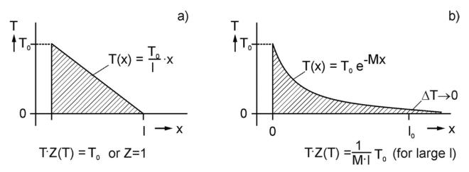
Fig.7 Linear versus exponential drop in temperature over the wire length T<sub>o</sub> maximal temperature.
