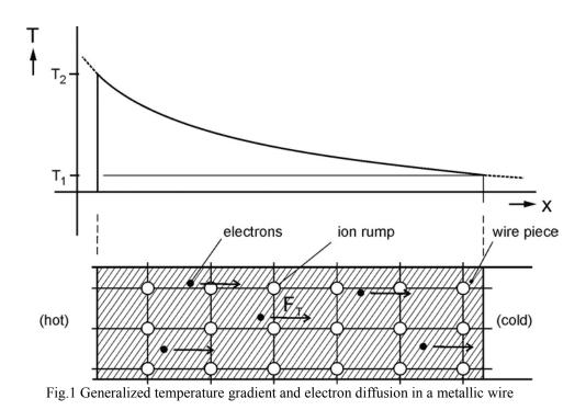
(4)  $F(T) = dW_e/dx$  or expanded by  $dT : F(T) = (dW_e/dT)(dT/dx)$
