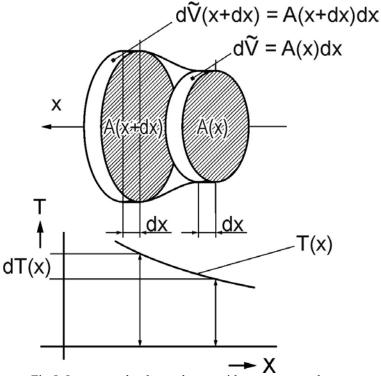
Fig.5: Incremental volume change with temperature change
