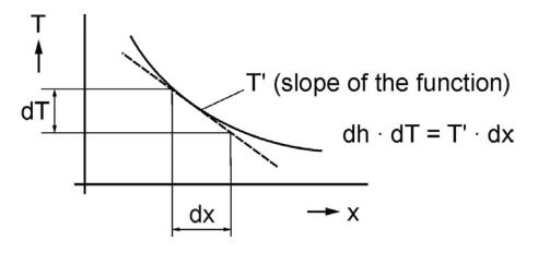
Fig.6: T(x) and its gradient.
