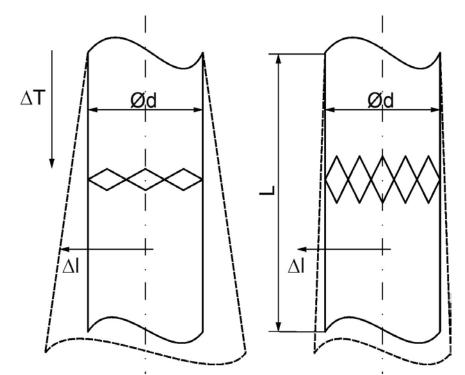
Fig.2 Uniaxial thermal expansion of thermoelectric materials, (a) short axis (b) long axis (c) table of  $\alpha$  and ASC values for different materials.
