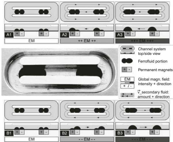
**Figure 1.** Ferrofluid-based generation of secondary fluid channel flow.
