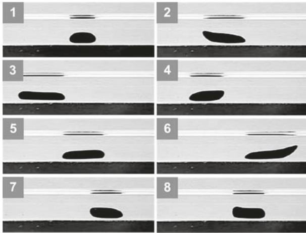
Figure 4. Active, uniaxial locomotion of a ferrofluid portion.
