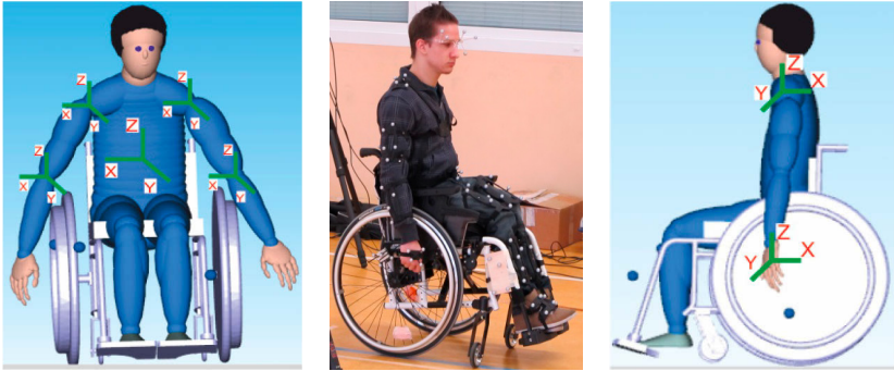
Figure 5.8 Position of the coordinate systems for investigating the motion of the wheelchair compared to the position of the markers
