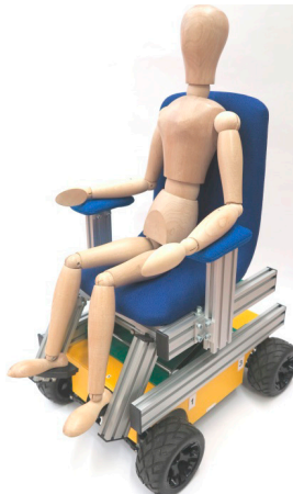
Figure 4.22 The front axle steerable platform – suitable for simple motion trajectories
