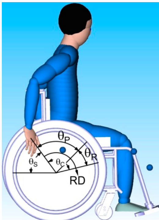
Figure 5.9 Important terminology for the analysis of motion capture
