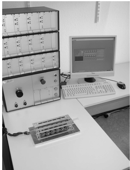
(b) Setup: module with coil arrangement and tunnel in front, plus computer-aided control of voltage-driven power supply.
