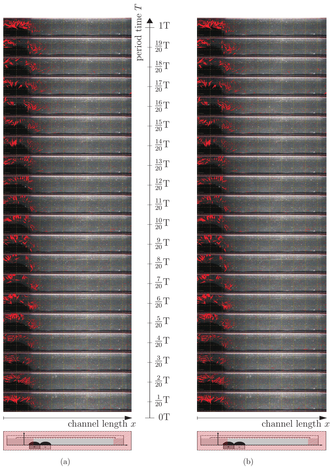
Figure C.13.: Traveling flow modes at (a) 12 Hz, and (b) 14 Hz excitation frequency.
