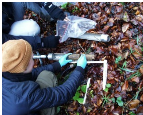
Fig. A17: Removal of soil from the split tupe in November 2005.
