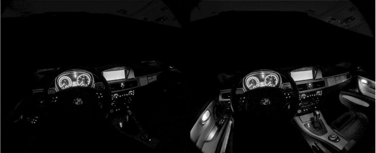
Figure 3.5 Experimental vehicle interior. Scenes without any ambient lighting (left) and with an ambient lighting scenario provided with centre console and doors illumination, including door handles and pulls (right). The instrumentation lighting is always turned on at a constant luminosity level. The display in the centre is on, showing a constant black screenshot.
