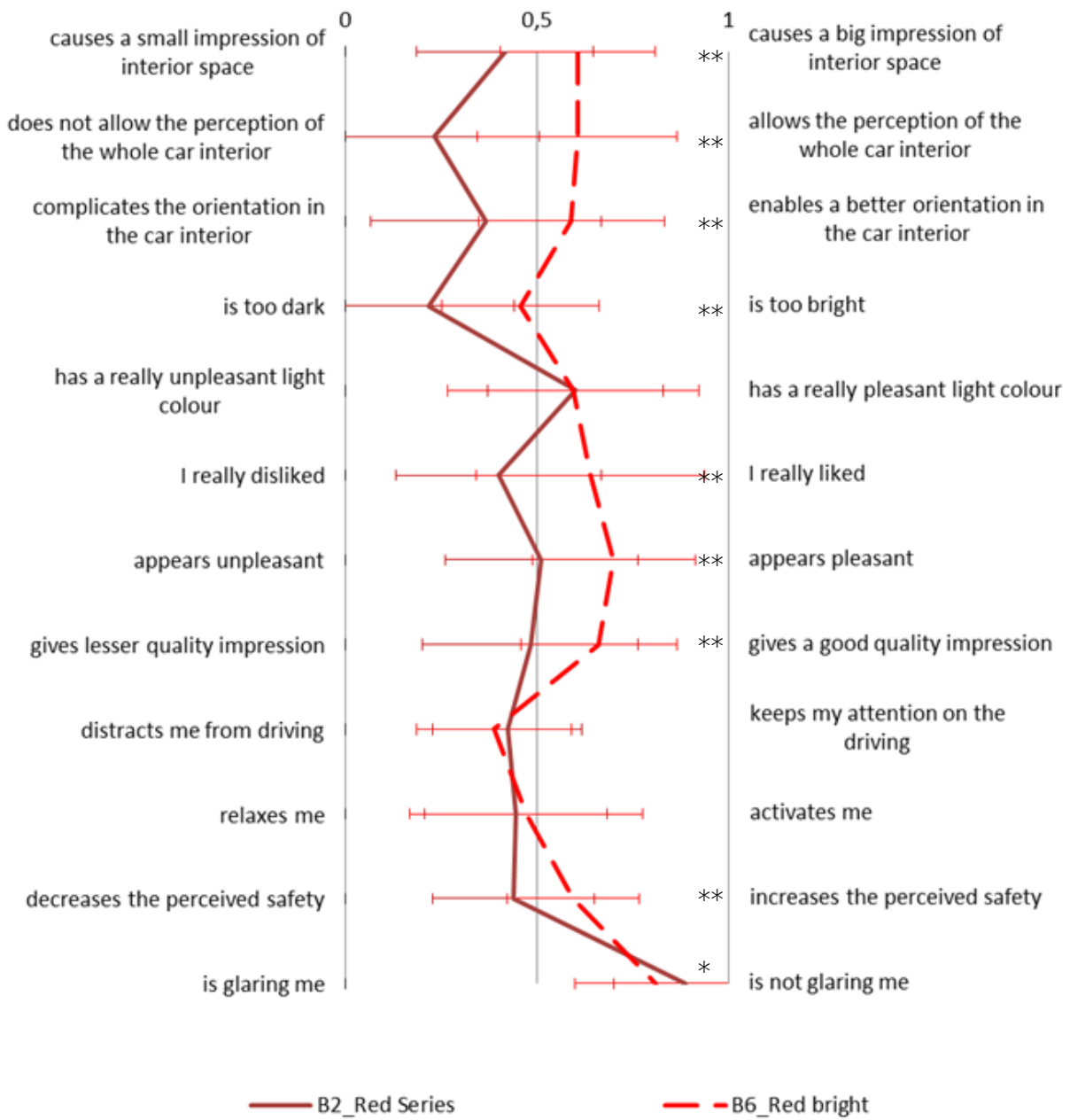
Figure 3.26 Results of the questionnaire of study B. The red scenarios series and bright are compared. For each question the mean value and the standard deviation of the answers are represented. * indicates a significant difference between the two results ( p < 0,05 ); ** indicates an high significant difference ( p < 0,01 ).
