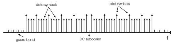
Figure 5.22: LDACS1 FL structure, one OFDM symbol in frequency domain [33].
