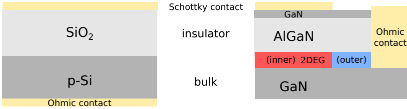
Figure 6.1: Structural comparison between a Si-based MIS and an AlGaN/GaN-MIHS
