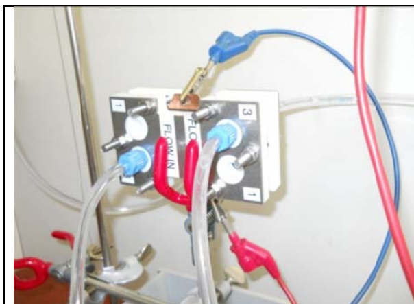
Figure 7.1 Electrochemical flow reactor for nitrate removal
