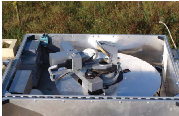
Figure 2.4: The Bruker Solar Tracker type A547 mounted in the custom made dome (shown in open state).
