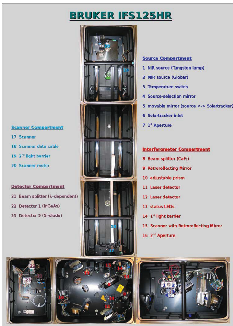
Figure 2.3: Illustration of the Bruker IFS125HR spectrometer and its components. The HCI cell was removed when the pictures were taken.
