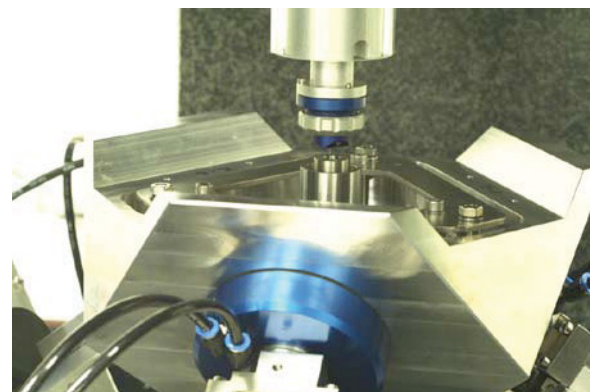
Figure 2. Moving workpiece table (aluminium dummy for testing purposes) supported by VPL air bearings.
