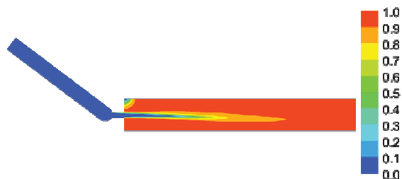
Figure 7: Volume fraction of diesel vapour (result of a not converged simulation)
