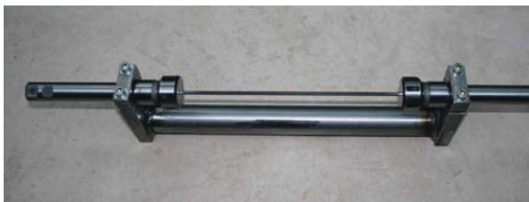
Fig. 7: Relaxation device for thin wires under torsional stress [3]
